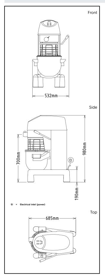
**Electric** Supply voltage: 200-240 V/1N ph/50/60 Hz Capacity: Performance (up to): 6 kg/Cycle 20 litres Capacity: **Key Information:**
